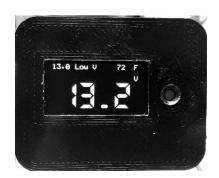
This display setting features a lowest sag detection self-resetting after 3 seconds, temperature reported by the IR sensor, and lastly the larger numerals indicating the current real-time voltage.
