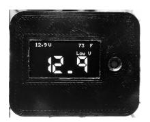
This display setting features the real-time voltage, temperature reported by the IR sensor, and lastly the larger numerals indicating the lowest sag detection that is self-resetting on a 3 second time interval.
