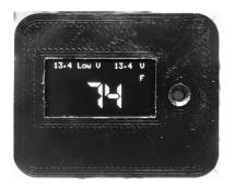
This display setting features a lowest sag detection self-resetting after 3 seconds, the real-time voltage display, and lastly a larger numerals indicating the temperature the IR sensor is reporting.
